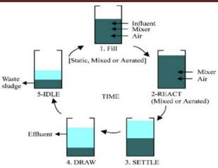
Fig.4: 5 Stages of Sequential Batch Reactor (SBR) Source: http://www.seamak.com/service\_6.html
